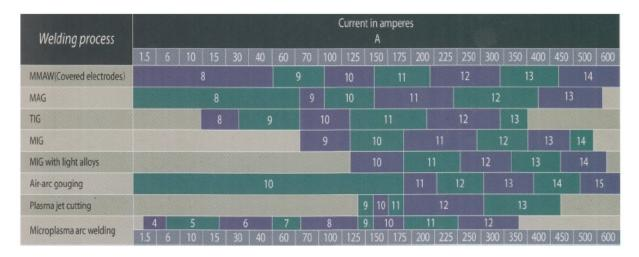
**Note:** The table recommends the most suitable welding filter darkening for various work applications. Slightly lower or higher values may be used depending on the conditions.
